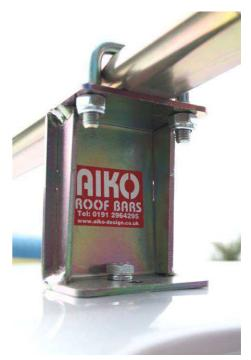
Put one longitudinal in place with the barest nip on the bolts- this will begin to align the cross bars...
