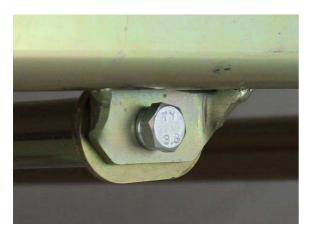
Again, the longitudinal bars are very straightforward- they bolt into the ends of the cross bars with an M8 x 16 bolt with a spring washer.
